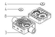
7. Replace sealing washers (4) The FT head does not contain a sealing washer or valve seats
