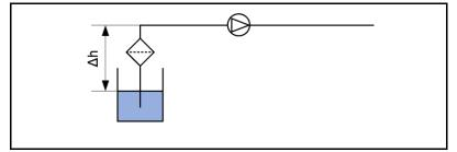
Fig. 18: Storage container underneath pump
