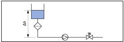
Fig. 19: Storage container above the pump.
