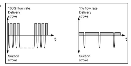
Fig. 5: Low-pulsation operating principle
