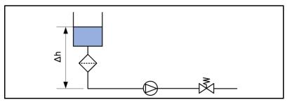
Fig. 68: Pressure test setup
