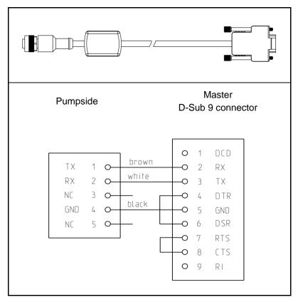
Fig. 65: KNF Flodos RC cable pin assignment
