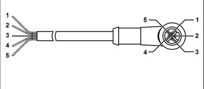
Fig. 53: KNF Flodos RC cable pin assignment
