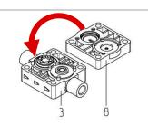
5. Fold the connecting plate (3) and the intermediate plate (8) apart
