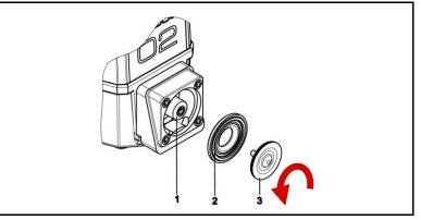
Fig. 67: Replacing the pump diaphragm
