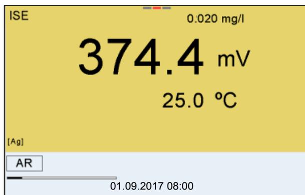
17. Wait for the end of the AutoRead measurement or accept the calibration value with <ENTER>.
