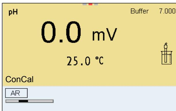
8. Wait for the measurement with stability control to be completed or terminate the stability control and take over the calibration value with <ENTER>.
