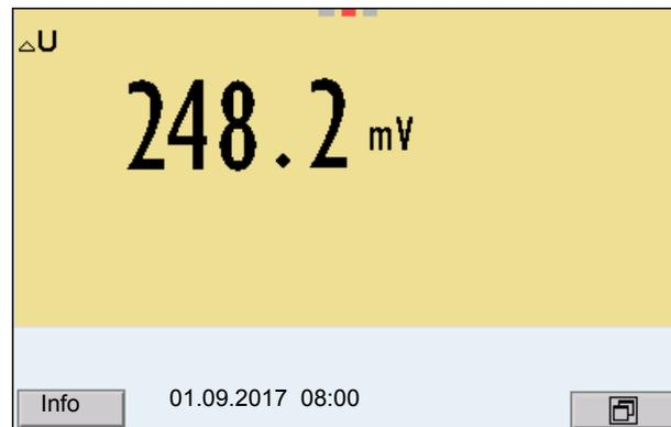
**AutoRead** The *Stability control* function checks whether the measured values are stable within the monitored time interval.
