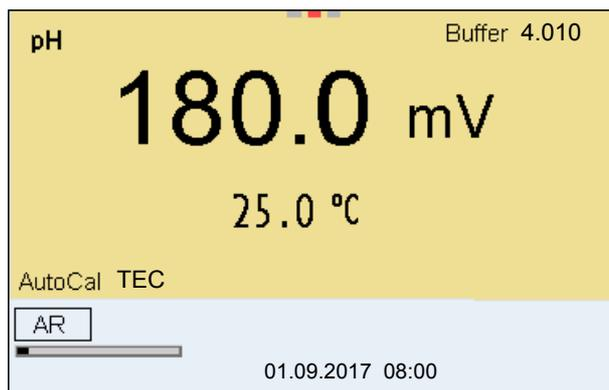
20. Wait for the measurement with stability control to be completed or terminate the stability control and take over the calibration value with **<ENTER>**.
