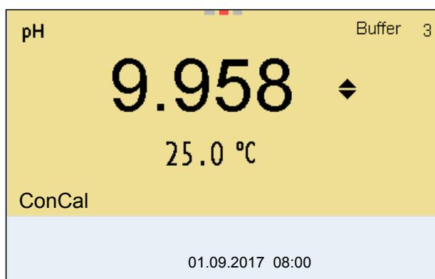
25. Set the nominal buffer value for the measured temperature with <▲><▼>.
