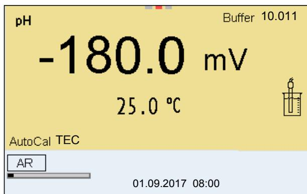
8. Wait for the end of the measurement with stability control or accept the calibration value with <ENTER>.
