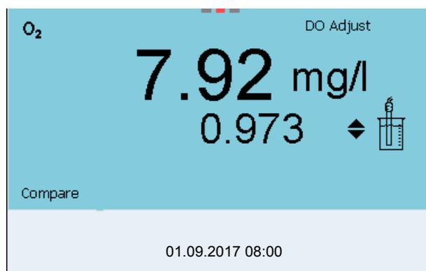
6. Using **<▲>** **<▼>**, set the correction factor to adjust the displayed concentration value to the nominal value (value of the comparison measurement). Subsequently, accept the correction factor with **<ENTER>**.
