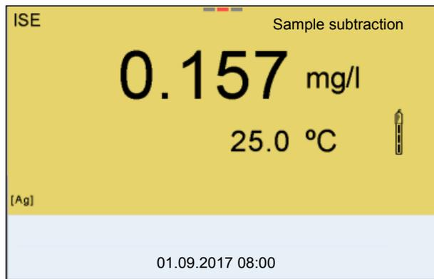
17. If necessary, start measuring further samples with **<ENTER>**. Repeat steps 8 - 16 for all samples.
