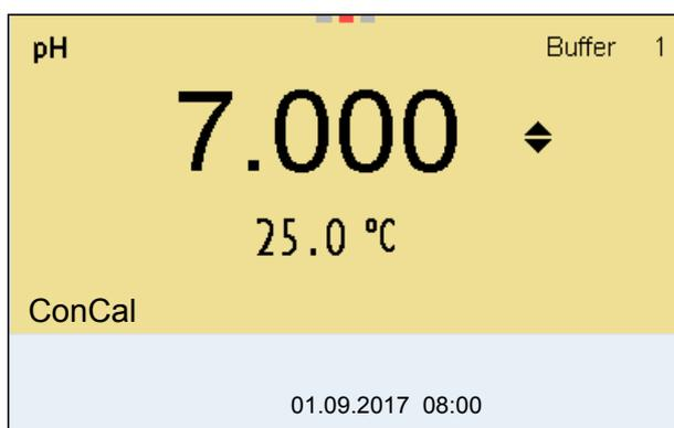
9. Set the nominal buffer value for the measured temperature with **<▲><▼>**.
