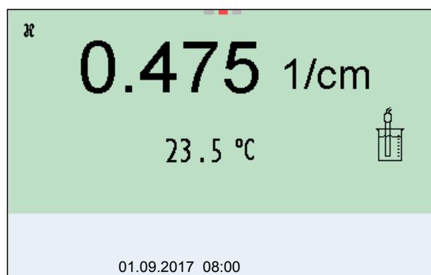
4. Immerse the conductivity sensor in the control standard solution, 0.01 mol/l KCl.
