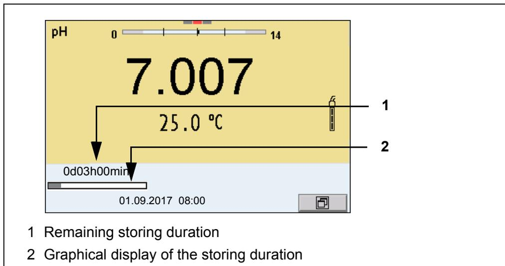
The active automatic data storing function can be recognized by the progress bar in the status line. The progress bar indicates the remaining storage duration.
