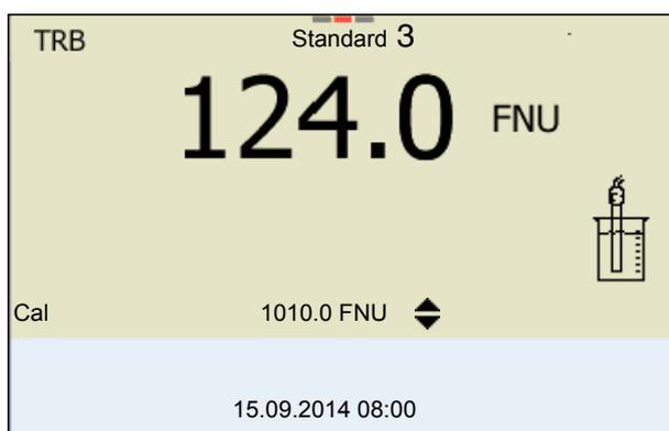
16. If necessary, terminate the calibration as a two-point calibration with **<M>**.
