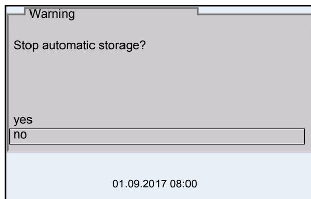
2. Using  $\langle \blacktriangle \rangle \langle \blacktriangledown \rangle$ , select *yes* and confirm with  $\langle \text{ENTER} \rangle$ .
