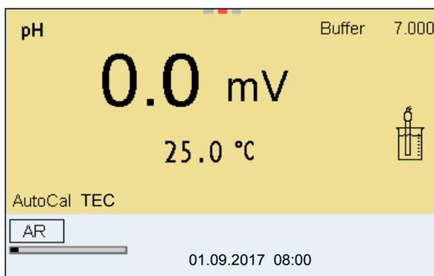
14. Wait for the measurement with stability control to be completed or terminate the stability control and take over the calibration value with <ENTER>.
