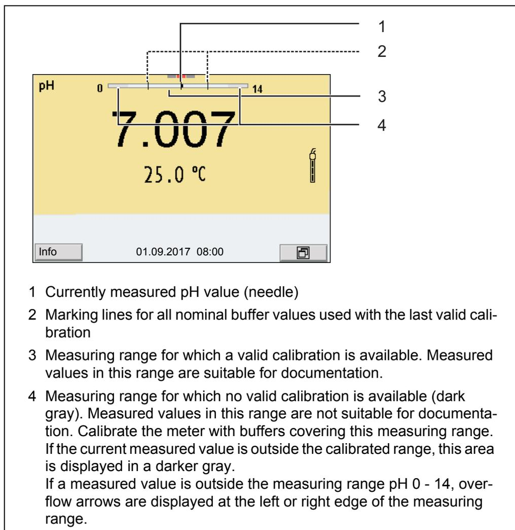
The limits of the calibrated range are determined by the buffers used for calibration:
