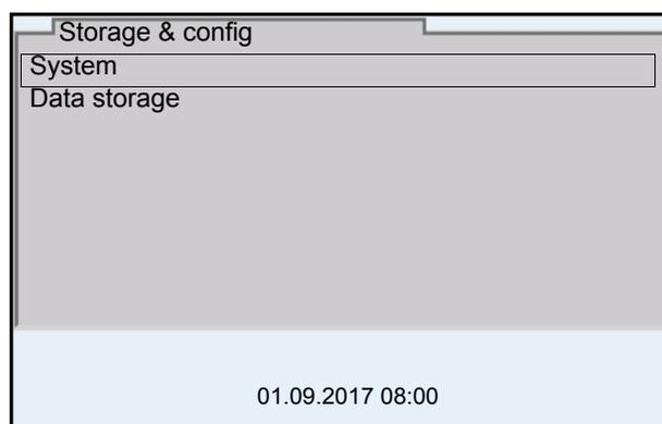
3. Select the *System* submenu with <▲><▼>. The current selection is displayed with a frame.
