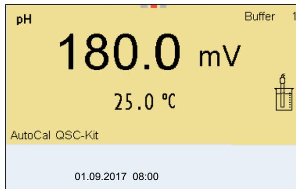
3. Calibration with the buffers of the QSC-Kit is done like a normal three-point calibration.
