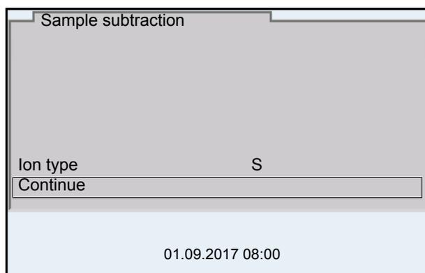
2. Using **<▲>** **<▼>** and **<ENTER>**, set the ion type for the ion in the standard (*Ion type*) as necessary.
