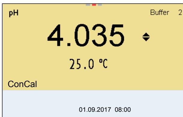
17. Set the nominal buffer value for the measured temperature with **<▲><▼>**.
