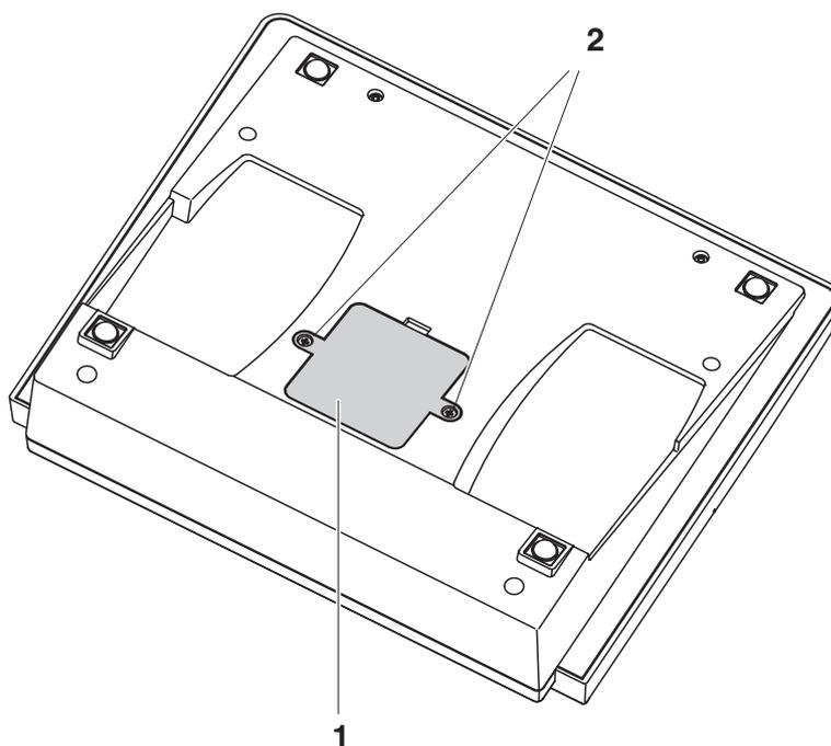
2. Open the battery compartment (1) on the underside of the meter.
