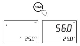
**Note:** The last measurement value will be displayed until the next sample is measured or the instrument is turned off. Temperature will be continuously updated.
