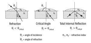
The critical angle can be used to easily calculate the refractive index according to the equation:
