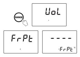
**Note:** The temperature measurement is not displayed in Freezing Point mode.
