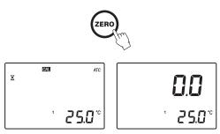
**Note:** The 0.0 screen will remain until a sample is measured or the instrument is turned off.
