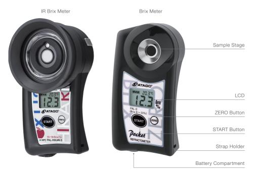
A combo set that includes PAL-HIKARi, a non-destructive IR Brix Meter that can measure the sugar content just by being pressed against the fruit, and a Brix meter that can measure the sugar content of squeezed fruit juice is now available.
