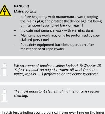
In stainless grinding bowls a burr can form over time on the inner edge between the bowl and the lid due to the ductility of the material. This burr causes the bowl and the lid to rest on each other, metal against metal, and the O-ring seal ceases to function. If you notice burr formation, it should be removed immediately with a scraper or fine emery paper before the burr becomes so large that removing it is difficult and requires a lot of effort.
