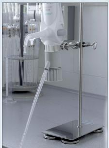
Stand clip for fixing the basic unit The stand clip also facilitates use of ceramus® in a stand assembly.
