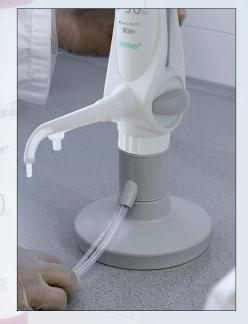
Base support instead of bottle attachment The base support enables suctioning of the medium directly from a separate storage con-
